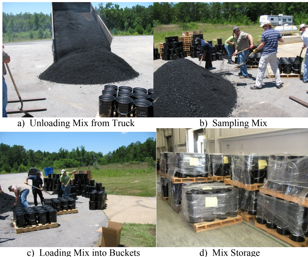
Figure 3.9 Mixture Sampling for Lab Testing
